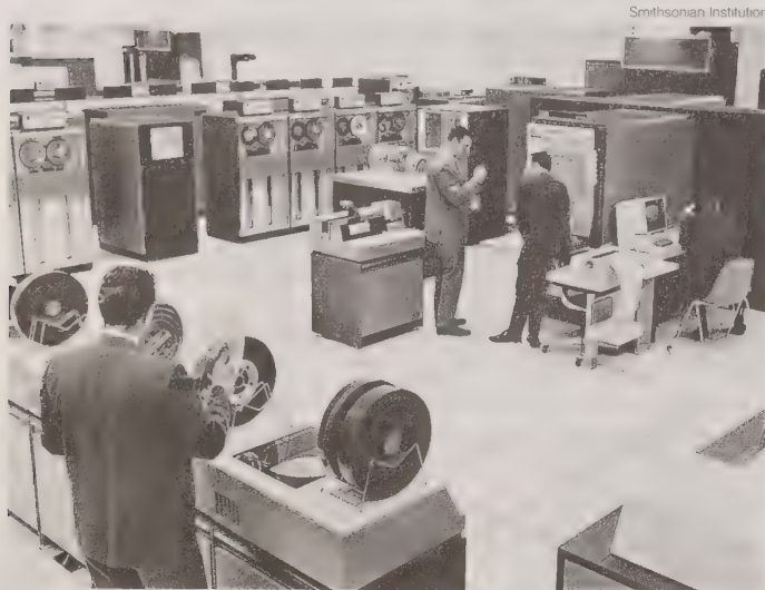
An IBM 360 computer, c. 1965. All machines in IBM's 360 line employed the same operating system, contributing to a flexibility that made it the definitive business computer of the 1960s.
